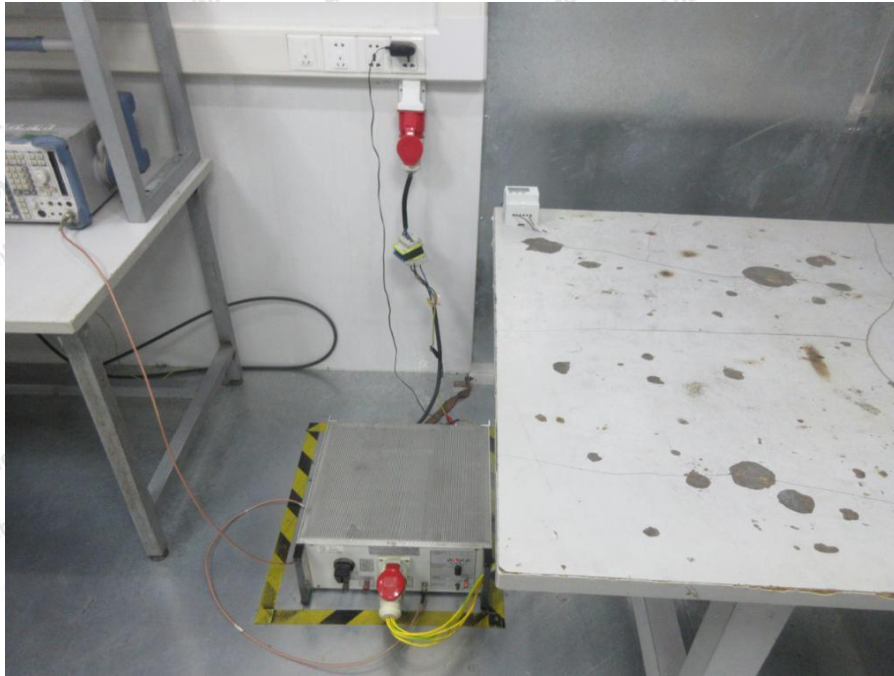
Photo of Power Line Conducted Emission Test
