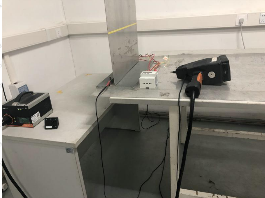
Photo of Electrostatic Discharge Immunity Test
