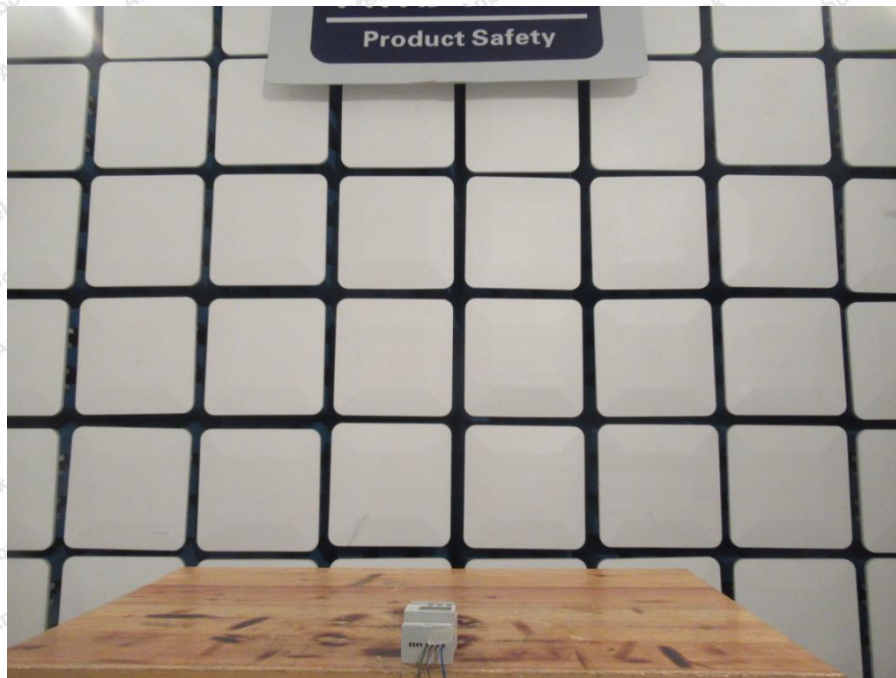
Photo of RF Field Strength susceptibility Test
