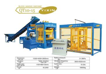
This QT10-15 automatic block making machine ,as the name shows, can make 10 blocks in dimension of 400\*200\*200mm with each mold .it is capable of making 16000 one day 8 working hours. In addition this product is able to make a variety of blocks or bricks with the variable molds.
