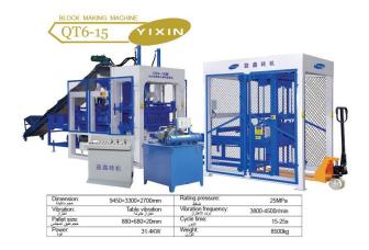
This QT6 automatic block making machine ,as the name shows, can make 6 blocks in dimension of 400\*200\*200mm with each mold .it is capable of making 9600 blocks or 200 to 120 cubic meters of blocks for one day 8 working hours. In addition this product is able to make a variety of blocks or bricks with the variable molds.
