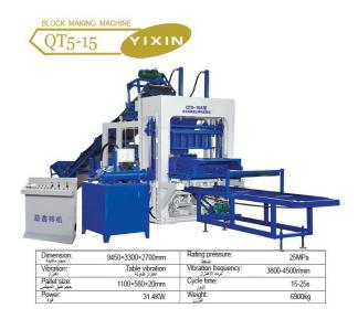
Seen from the model number of the QT5-15automatic block making machine, the product is capable of making 5 blocks in size of300\*200\*100mm by each mold and the operation cycle lasts 20 seconds. Additionally, our product has the production capacity of 8000 blocks within 8 working hours. Due to the changeable molds, this automatic block making machine is available in forming diversified blocks, bricks and other products.
