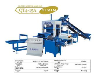
Seen from the model number of the QT4-15automatic block making machine, the product is capable of making 4 blocks in size of 400\*200\*200mm by each mold and the operation cycle lasts 20 seconds. Additionally, our product has the production capacity of 1600blocks within 8 working hours. Due to the changeable molds, this automatic block making machine is available in forming diversified blocks, bricks and other products.
