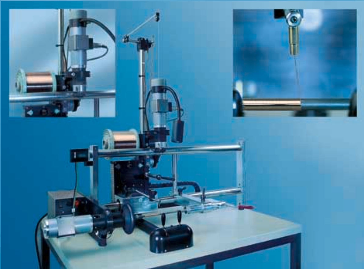
special machinery for isocyclic winding of coils
