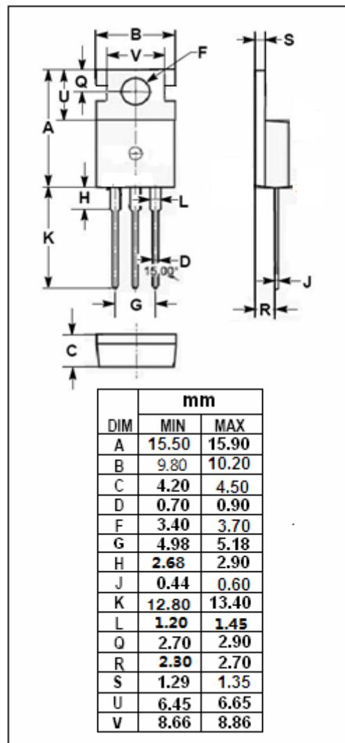
**isc Three Terminal Positive Voltage Regulator****7805****• ELECTRICAL CHARACTERISTICS** $T_j=25^\circ\text{C}$  ( $V_i=10\text{V}$ ,  $I_o=0.5\text{A}$ ,  $C_i=0.33\mu\text{F}$ ,  $C_o=0.1\mu\text{F}$  unless otherwise specified)
